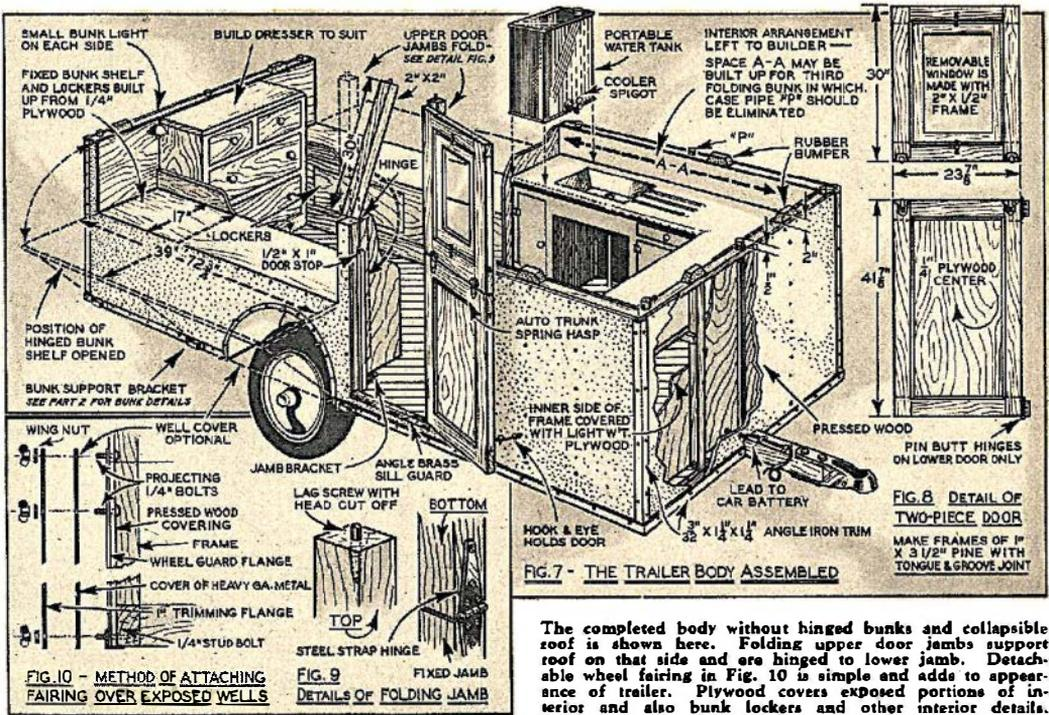
The completed body without hinged bunks and collapsible roof is shown here. Folding upper door jambs support roof on that side and are hinged to lower jamb. Detachable wheel fairing in Fig. 10 is simple and adds to appearance of trailer. Plywood covers exposed portions of interior and also bunk lockers and other interior details.
