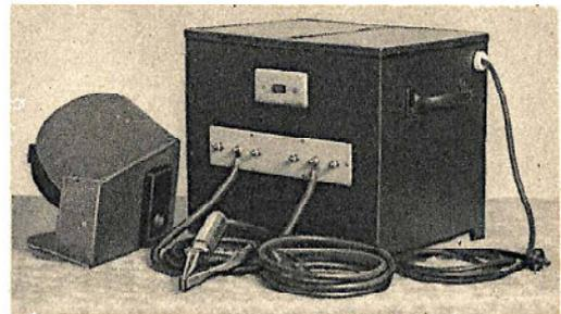
Electric arc welder operates without interruption. High frequency current maintains connection between electrode and work. Shield protects face from ultra-violet sunburn.
