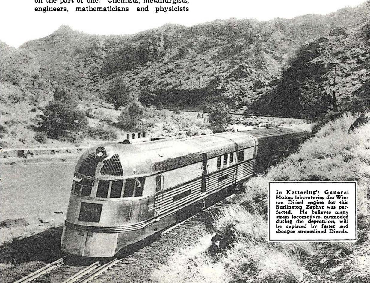
In Kettering's General Motors laboratories the Winton Diesel engine for this Burlington Zephyr was perfected. He believes many steam locomotives, outmoded during the depression, will be replaced by faster and cheaper streamlined Diesels.
