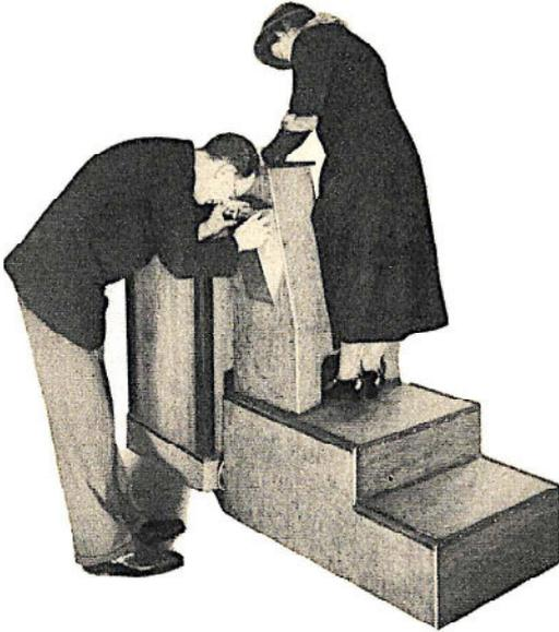
The customer puts foot through hole in machine and looks through the view plate to see how the shoe fits the foot.
