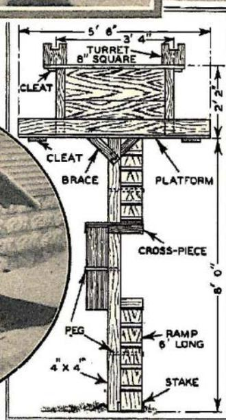
Little bits of meat placed on cleats of ramp will entice your dog up to this pup penthouse the first time; after that he'll thoroughly enjoy climbing ramps to reach the breezy platform. Platform and house are square, with necessary dimensions for small dog given at right. Cover roof with tar paper; small slant here will help water to drain off. Make ornamental door and nail open as shown. House and ramp must be strong and well-braced.
