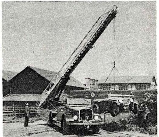
Fire ladder, used as a crane, rescues automobile after wreck.
