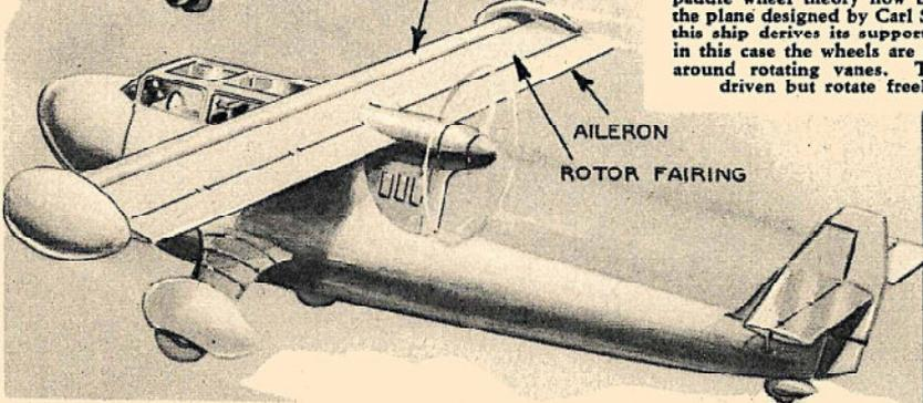
The ship at left, designed by Alexander Chessin and Serge Trey, is intended to improve safe flying. A 12-inch hollow cylinder, 23 feet long forms the leading edge of the wing. Built on the Flettner rotor principle, it rotates 7,000 r.p.m. A constant stream of air is directed onto the cylinder by tiny jets to insure continuous lift.
