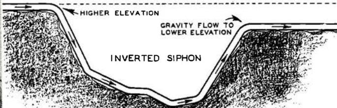
Inverted siphons like that above are not true siphons. Water finds its own level after plunging to bottom of canyon. Friction accounts for small loss in elevation. This construction is being used by Metropolitan Water District of Southern California in construction of Colorado River Aqueduct, to take place of flumes or arch supported structures crossing canyons.
