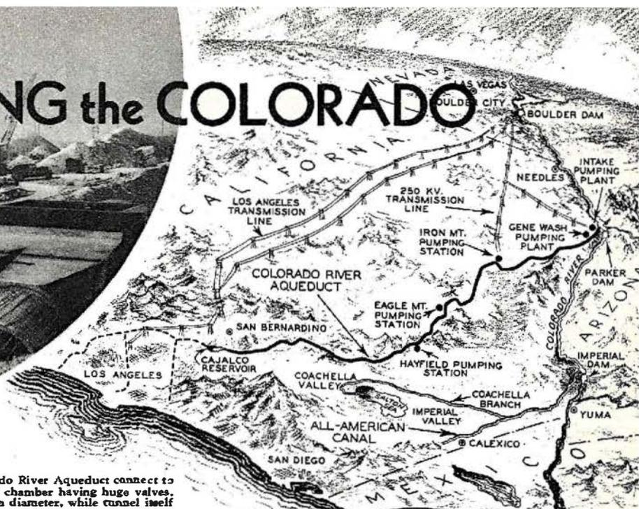
Double siphons of Colorado River Aqueduct connect to tunnels through transition chamber having huge valves. Each "barrel" is 12 feet in diameter, while tunnel itself is 16 feet in diameter. Map at right shows how all four projects are related to each other and to Boulder Dam.
