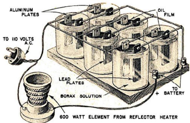
Construction of heavy duty electrolytic charger is shown above. Aluminum plates will gradually wear away, and may need replacement. Size of plates determines current which will pass; thickness determines life of plates. Pour film of clean oil over solution in each jar to prevent evaporation. Iron or copper may be used in place of lead. Baking soda ( $\frac{1}{2}$  oz. to gallon of water) works as well as borax. Current density is about 100 ma. per sq. in. of immersed aluminum surface.
