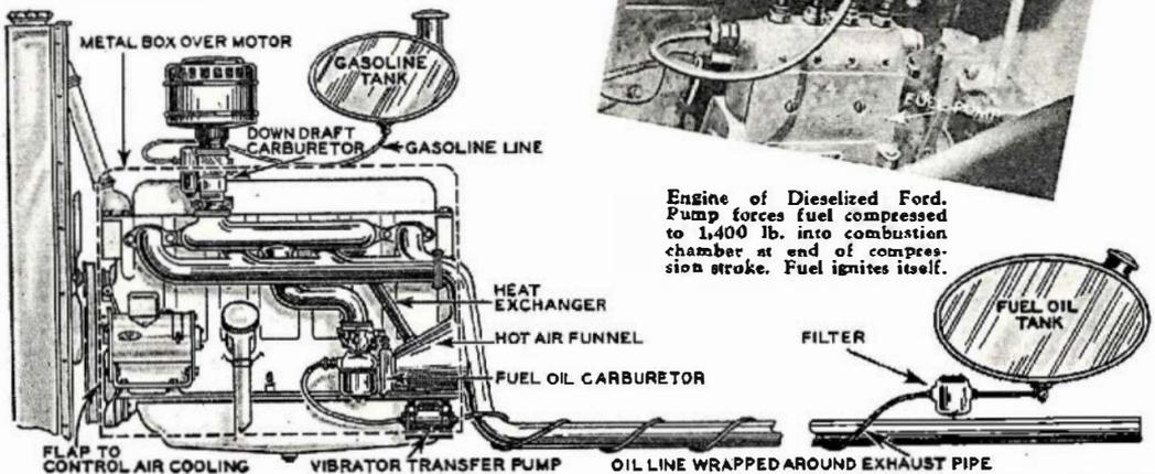
Drawing indicates changes made by Don Redman in 1930 Chevrolet to permit use of either gasoline or fuel oil. Entire installation cost less than \$15. Jets of original carburetor are altered, and this used for fuel oil. New down-draft carburetor is added as shown, to vaporize gasoline. Dual throttles and carburetors make the switch from gas to oil almost instantaneous.
