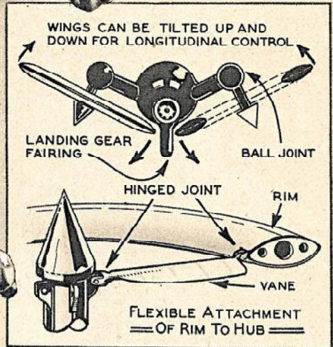
The "Spinning Top" plane, illustrated in the drawings above, is the latest idea for the application of the paddle wheel theory now being tested abroad. Like the plane designed by Carl Strandgren (at left above), this ship derives its support from rotating wheels but in this case the wheels are composed of an outer rim around rotating vanes. The vanes are not power driven but rotate freely as in the autogiro.
