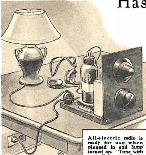
All-electric radio is ready for use when plugged in and lamp turned on. Tune with top dial, control regeneration with lower dial shown on the panel.
