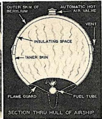
Hot air furnishes the lifting power for this newly-designed dirigible. Cross-section of hull (above) reveals inventor's unique method of using fuel for warming the inside area of the giant bag.
