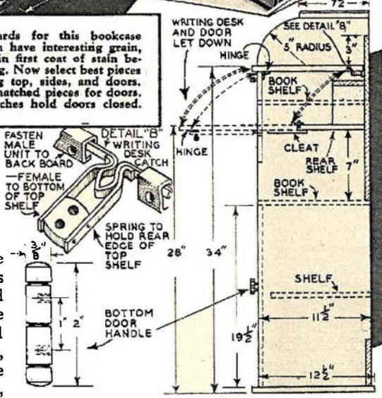
Build your desk to dimensions shown above. Special spring catch holds writing desk in closed position. Small turn-buttons of brass, like those used on window screens, hold desk in open position for writing. Door handles are turned from 3/8" brass rod. Drill mounting holes with No. 33 drill, tap with No. 6-32, and use 6-32 screws. Use brass tubing as spacers over bolts. Lacquer all hardware to retain lustr.
