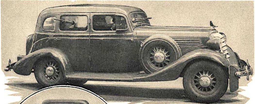
Above—A side view of car showing gun ports in windows. Left—Bulletproof screens protect the tires and radiator.
