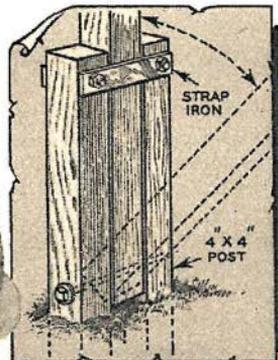
Annual cleaning of bird houses on tall poles is easier if this pivoted mounting is used. House can then be taken down for winter storage, easily set up again in spring. Support post pivots between two 4"x4" uprights sunk into ground, a  $\frac{3}{4}$ " bolt going through all three pieces. To tilt support post, simply remove one of iron straps bolted to the tops of uprights.
