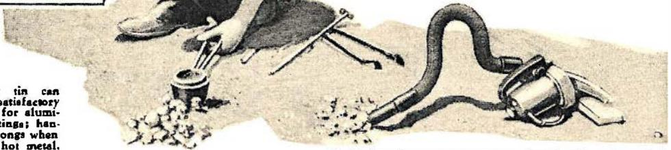
**B**RASS, bronze, or aluminum castings for model projects or even larger work can be made in your own "hole-in-the-ground" foundry at a cost of no more than one cent each--castings so accurate, so smooth that they are ready for use after only a few minutes on the buffing wheel.
