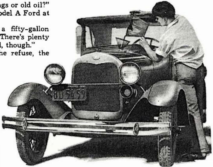
Tank of this Dieselized Model A Ford is filled with crankcase drainings, not gasoline. In towing large car from Phoenix to Los Angeles, driver made 26 miles per gallon of fuel oil.
