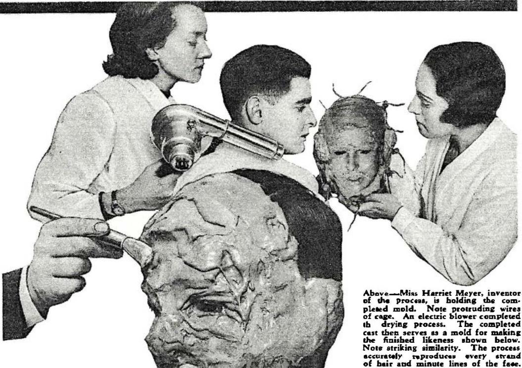
Above—Miss Harriet Meyer, inventor of the process, is holding the completed mold. Note protruding wires of cage. An electric blower completed the drying process. The completed cast then serves as a mold for making the finished likeness shown below. Note striking similarity. The process accurately reproduces every strand of hair and minute lines of the face.
