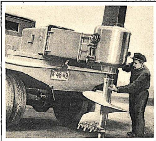
In order to speed their tree-planting program, Moscow engineers devised above machine to dig the holes for planting.
