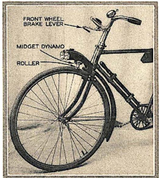
Above photo shows bike light installed. The roller rests against the tire and spins to generate current for light.
