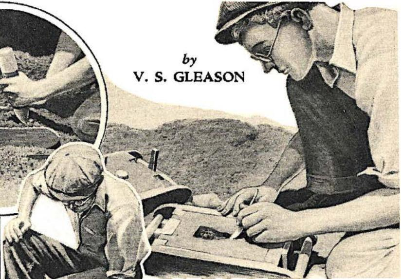
Scoop out channel with spoon from pouring hole to casting impression in drag. Note notches at ends of drag, and aligning pegs on cope which insure accuracy of mold. Metal rod seen on cope is removed, leaving gas-escape hole.
