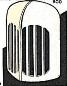
FIG. 8 BRASS BARS, SOLDERED IN, NICKEL PLATED
