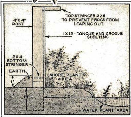
The best type of fence for frog farms is a solid wood structure built as shown above to prevent frogs from leaping out.
