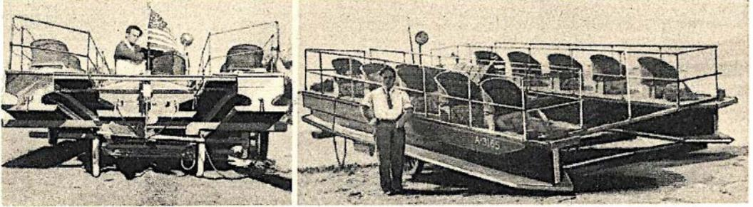
Left—Rear view of newly-built pontoon speed boat. Note the anti-wave-splash grooves which, dipping downward, tend to buoy up the stern. Right—Chairs for passengers are placed atop the framework into which the power unit nests.
