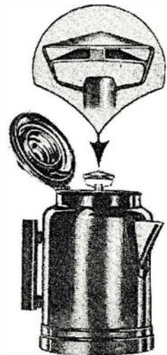
Simple deflector slips over percolator pipe, prevents cracking of the glass top.
