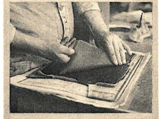
Above photos follow the method of preparing the rubber plates. Respective steps are shown from upper left to lower right. The mat is carefully glued to plate glass after which the rubber composition is poured on in even layers. It is smoothed carefully with fingers to insure perfect impression and the back is leveled. After setting, it is baked in an oven until hardened. Then it is removed, the mat peeled off and plate is ready for printing.
