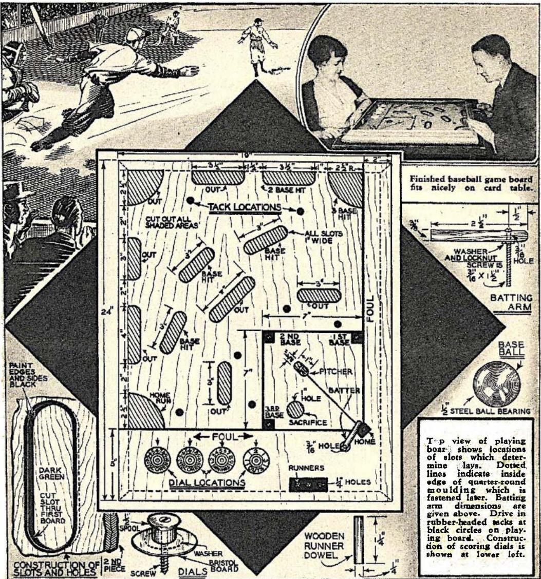
moulding to the blocks all around the board to form the sides. The plywood pieces are now fastened together with small screws around the edges. Nail a piece of wallboard to the blocks for a bottom covering.
