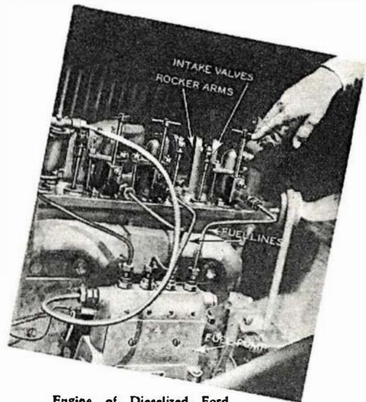
Engine of Dieselized Ford. Pump forces fuel compressed to 1,400 lb. into combustion chamber at end of compression stroke. Fuel ignites itself.
