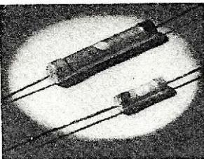
Lead wires are firmly attached to ends of improved type radio resistor having constant characteristics, high current carrying capacity. Color code indicates size.
