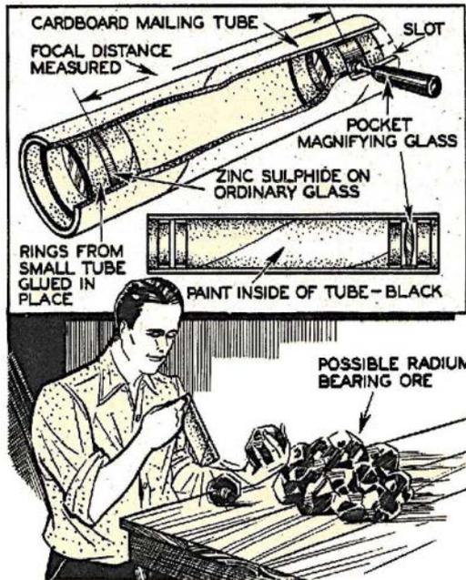
Zinc sulphide, sprinkled over adhesive on window glass end, glows when held over radium bearing ore in a dark chamber.
