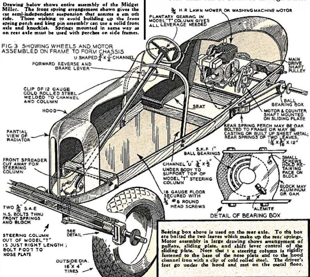
Bearing box above is used on the rear axle. To the box are bolted the two leaves which make up the rear springs. Motor assembly in large drawing shows arrangement of pulleys, sliding plate, and shift lever control of the sliding plate. Note that the steering column is rigidly fastened to the base of the nose plate and to the hood channel iron with a clip of cold rolled steel. The driver's feet go under the hood and rest on the metal floor.
