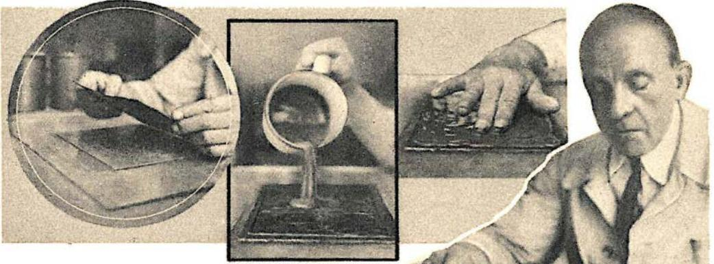
**N**EWSPAPER presses throughout the country, roaring along at top speed, will soon be able to roll off colored sections, comics and pictures with unusually sharp detail, using rubber plates for direct printing in place of ordinary metal plates. Developed recently in Germany, such fine screen rubber half-tones, employing a minimum of printing ink, are able to make a satisfactory impression on almost any kind of surface without the usual makeready.
