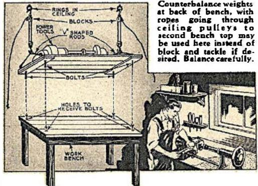
Counterbalance weights at back of bench, with ropes going through ceiling pulleys to second bench top may be used here instead of block and tackle if desired. Balance carefully.
